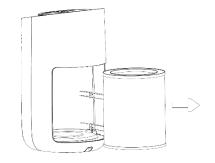
2. Push the filter down and twist it clockwise to remove.
